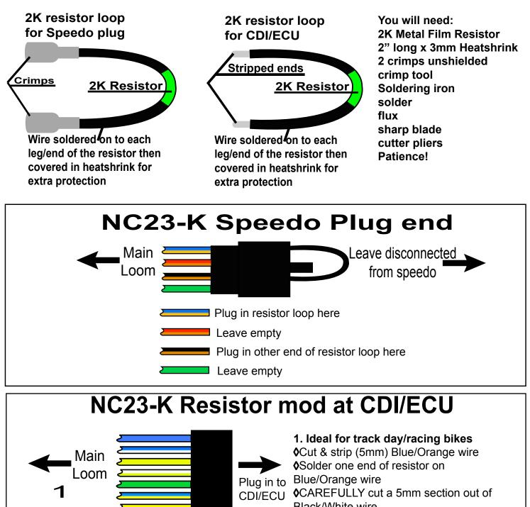
Black/White wire Solder other end of resistor on to Black/White wire section
