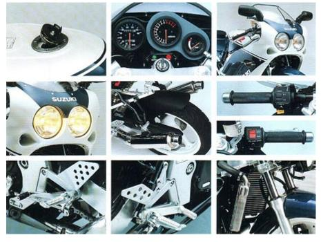
The GSX-R400 got a new frame (GK73A) and new overall appearance in 1988. The new model was presented in February 1988. The redesigned GSX-R got once again new fairing and shorter wheelbase, but the weight increased a bit due to the stronger new chassis and exhaust system. The model also got slingshot carburetors, polished chrome silencers, curved radiator, Tokico 4-cylinder front brake calipers and a rear hugger mudquard.
